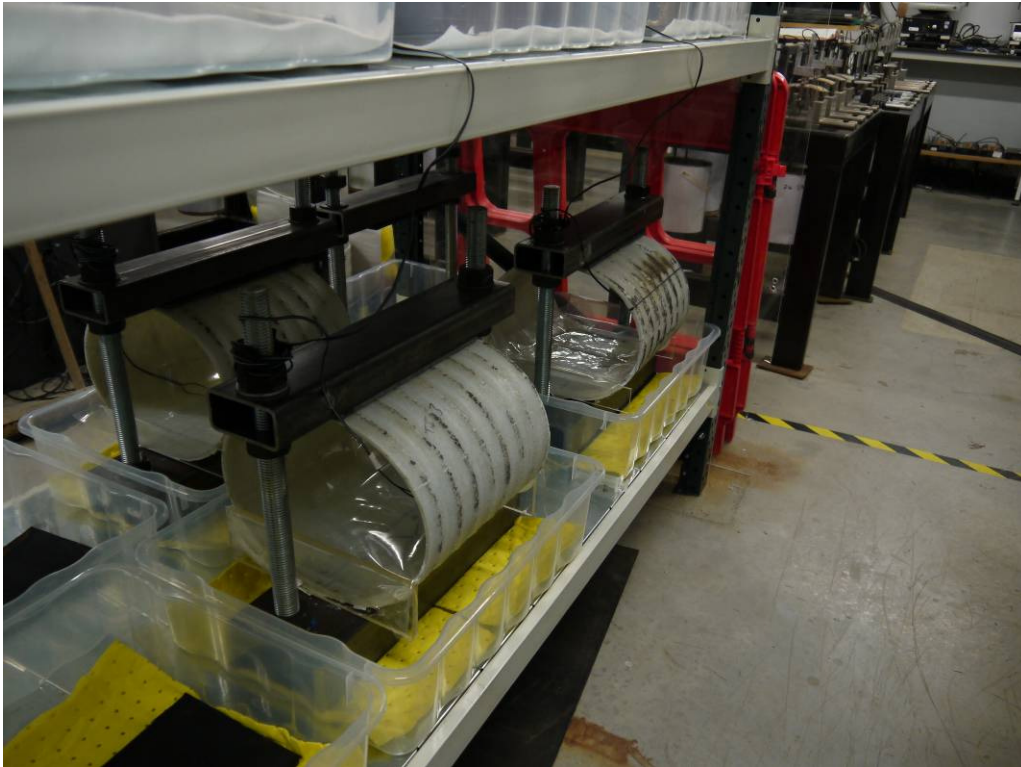
Figure 1, example photograph showing strain corrosion test set-up
